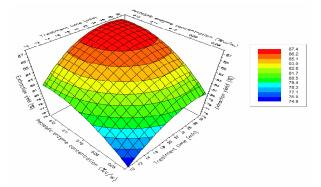
Figure 3. Response surface plot for extraction yield in the simultaneous treatment of acelora mash by ultrasound and pectinase preparation
